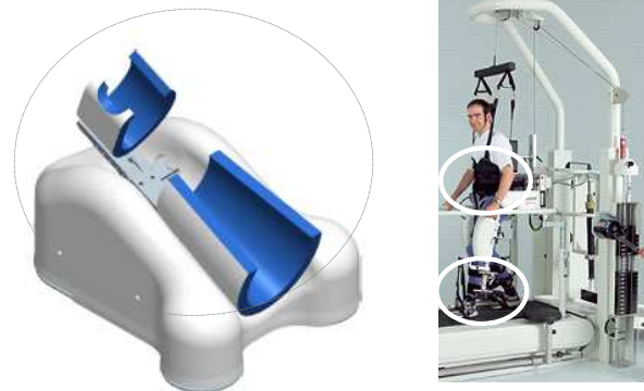
Figure 1. ArmAssist [1] (left) and the Lokomat [2] (right). The limb attachment or connective parts that are encircled in these pictures are the topic of this paper.
